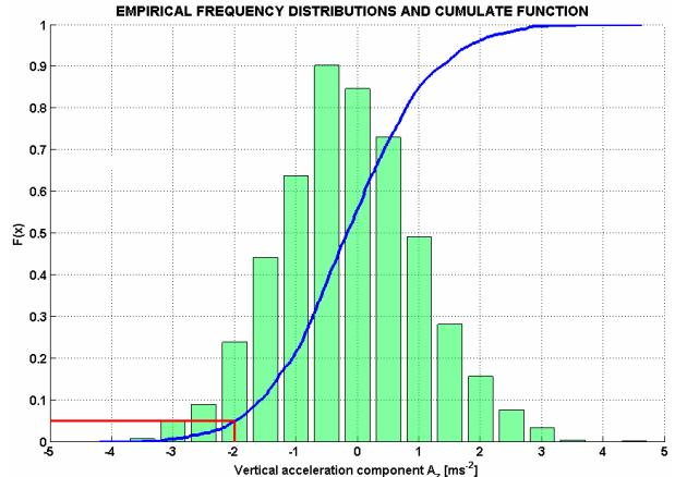
Figure 3. Vertical acceleration distribution and cumulate function.
