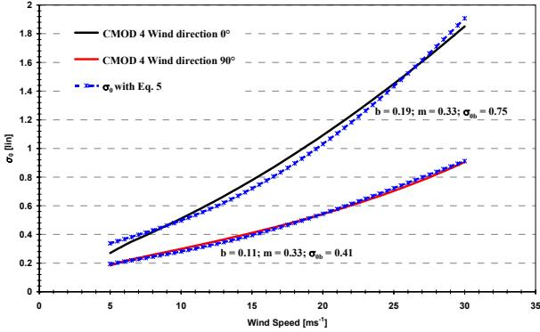
Figure 1. CMOD-4 Radar Equivalent Cross Section for  $\theta = 23^\circ$ ; wind direction  $0^\circ$  and  $90^\circ$ . Eq. 5 for range travelling waves ( $b=0.19$ ,  $m=0.33$ ,  $\sigma_{ob}=0.75$ ) and for azimuth travelling waves ( $b=0.11$ ,  $m=0.33$ ,  $\sigma_{ob}=0.41$ ).
