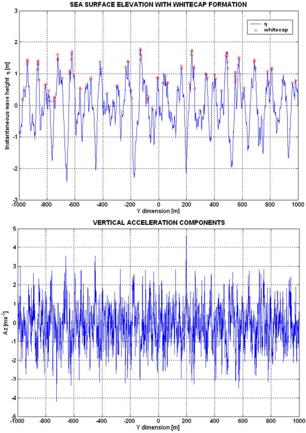
Figure 4. Water elevation and acceleration map. Simulated whitecaps are marked with red circles.
